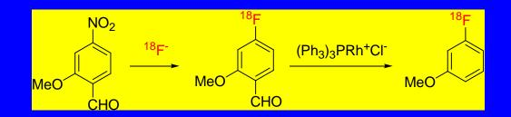
This constitutes a two-step procedure for introducing NCA [<sup>18</sup>F]fluoride into non-activated (electron-rich) rings
