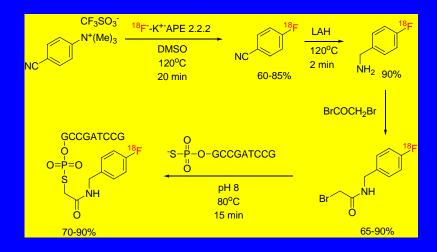
Overall radiochemical yield:: 40%( decay-corrected)Preparation time: 220 min
