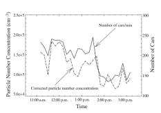
**Figure 2.** Correlation between traffic density and measured total PN concentration, corrected for wind velocity, 30 m downwind from the freeway. Reprinted with permission from Zhu et al. (2002b). Copyright 2002 Air and Waste Management Association.
