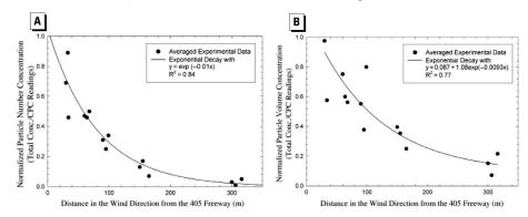
**Figure 1.** Normalized total particle (*A*) number and (*B*) volume concentration, in the size range of 6 –220 nm, as a function of distance from the I-405 freeway. CPC, condensation particle counter (TSI Inc., Shoreview, MN). Reprinted with permission from Zhu et al. (2002b). Copyright 2002 Air and Waste Management Association.
