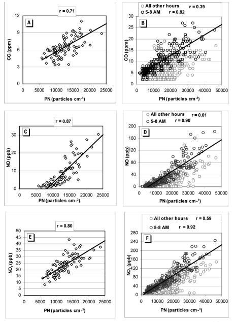
**Figure 9.** PN concentrations vs. CO, NO, and NO<sub>2</sub> in Riverside, California, during summer 2002. (*A*) 24-hr average PN vs. CO, (*B*) hourly PN vs. CO, (*C*) 24-hr average PN vs. NO, (*D*) hourly PN vs. NO, (*E*) 24-hr average PN vs. NO<sub>2</sub>, (*F*) hourly PN vs. NO<sub>2</sub>. Reprinted with permission from Sardar et al. (2004). Copyright 2004, Air and Waste Management Association.
