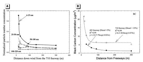
**Figure 4.** (*A*) Normalized PN concentration for different size ranges as a function of distance to the I-710 freeway. (*B*) Concentrations of BC as a function of distance from the I-405 and I-710 freeways. Reprinted from Zhu et al. (2002b). Copyright 2002, with permission from Elsevier.
