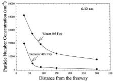
Figure 6. Comparison of decay of PN concentrations in summer and winter in the size range of 6–12 nm near the I-405 freeway. Reprinted from Zhu et al. 2004: "Aerosol Science & Technology: Seasonal Trends of Concentration and Size Distribution of Ultrafine Particles Near Major Highways in Los Angeles." 38(suppl 1):5–13. Copyright 2004. Mount Laurel, NJ. Reprinted with permission.
