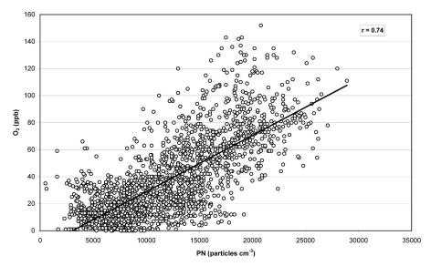
**Figure 10.** Hourly PN vs.  $0_3$  concentrations in Glendora, California, during summer 2002, with a lag time of 2 hr (PN vs.  $0_3$  2 hr earlier). Reprinted with permission from Sardar et al. (2004). Copyright 2004, Air and Waste Management Association.
