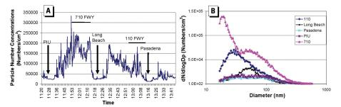
**Figure 8.** In-vehicle measurements of (*A*) PN concentrations (*B*) number-based particle size distributions, in freeways and urban areas in Los Angeles, CA. PIU, particle instrumentation unit, located at the southern California Supersite in downtown Los Angeles. Long Beach and Pasadena are two other urban areas in Los Angeles. Arrows indicate when the vehicle was off road at these three urban locations. From Westerdahl et al. (2005). Copyright 2005, with permission from Elsevier.
