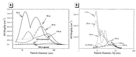
Figure 3. UFP size distribution at different sampling locations near (*A*) the I-405 freeway [reprinted with permission from Zhu et al. (2002b); copyright 2002 Air and Waste Management Association] and (*B*) the I-710 freeway [reprinted from Zhu et al. (2002a); copyright 2002, with permission from Elsevier].
