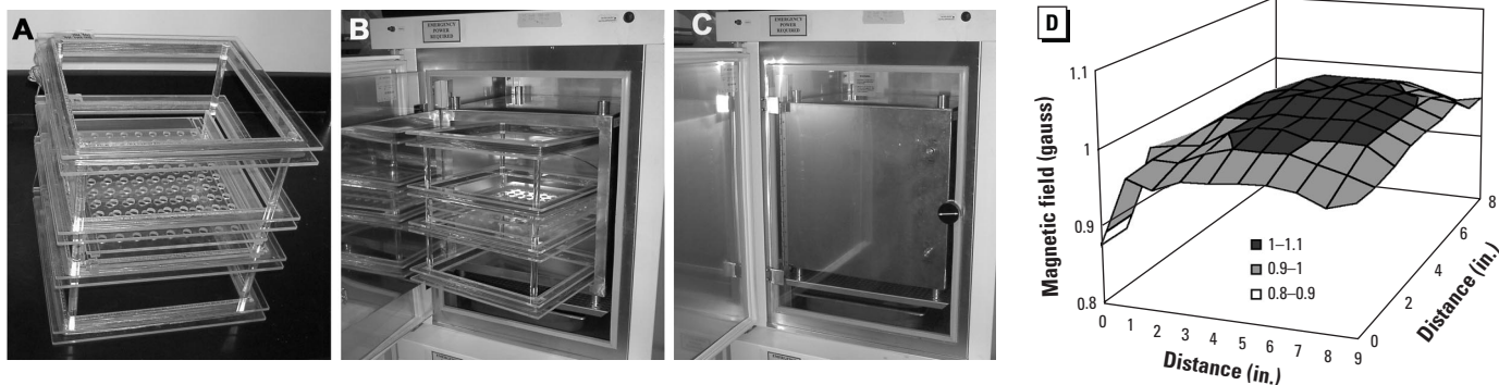
Figure 1. EMF exposure system and field distribution. (A) Photograph of cube-shaped Merritt coil. (B) Photograph of the coil inside the mu-metal box, which was placed inside a CO 2 incubator. (C) Photograph of the mu-metal box inside the CO 2 incubator. (D) Magnetic field distribution within the closed mu-metal box when a 100 \mu T (1 gauss) field was applied in the coil. The central region of about 25 square inches was very uniform, and this was where culture plates were positioned. See “Materials and Methods” for details.
