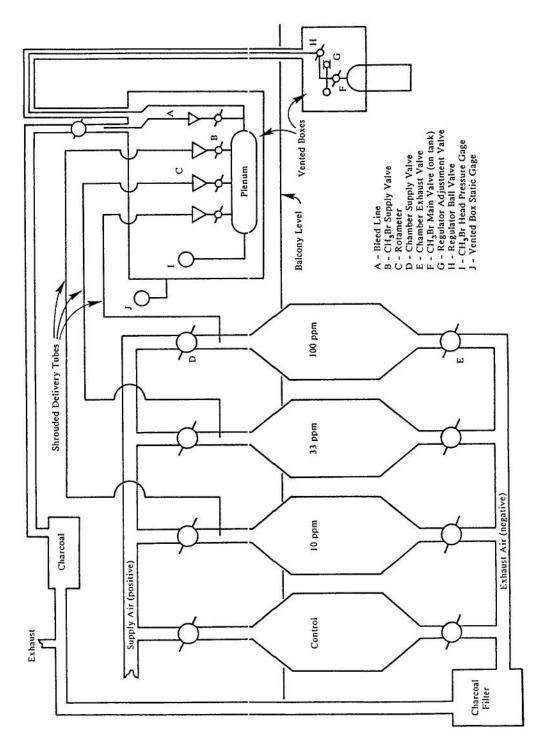
FIGURE G3 Generation System for Methyl Bromide
