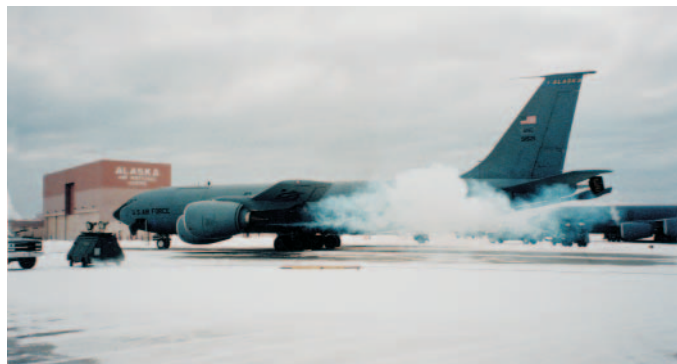
Figure 1. Typical exhaust plume from an engine run-up procedure for a KC-135 aircraft in a cold climate (-10°C). During aircraft warm up, the exhaust contains unburnt and partially burnt JP-8, exposing crew chiefs and other ground personnel to JP-8. During multiple-aircraft starts, a low-hanging exhaust cloud may form over the whole tarmac area.
