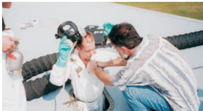
Figure 2. Fuel tank entry worker exiting wing tank of a C-141 aircraft after routine maintenance procedures. Immediately after removing his forced air respirator, the subject provides a postexposure breath sample.
