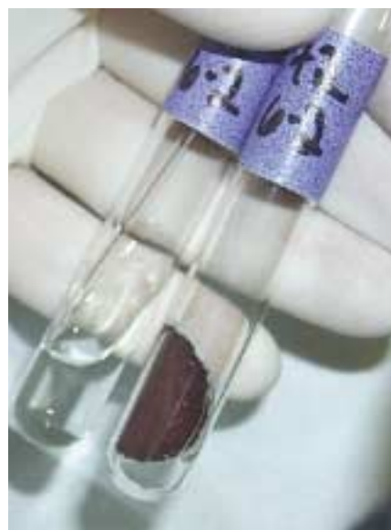
Figure 2. Blood spot extraction. Whole blood spots are extracted overnight in 2 mL methanol. The methanol containing extracted PbTx-3 is removed and blown to dryness with N 2 for analysis on receptor-binding assay or by LC-MS/MS. This extraction method provides a quick and simple method to separate brevetoxin from the blood matrix.
