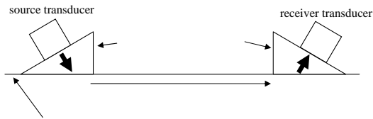
Figure 2. Schematic of the ultrasonic wave speed measurement.
