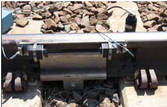
Figure 5. Magnetically attached ultrasonic wave speed measurement device shown attached to the outer surface of the rail head at a stress module location.
