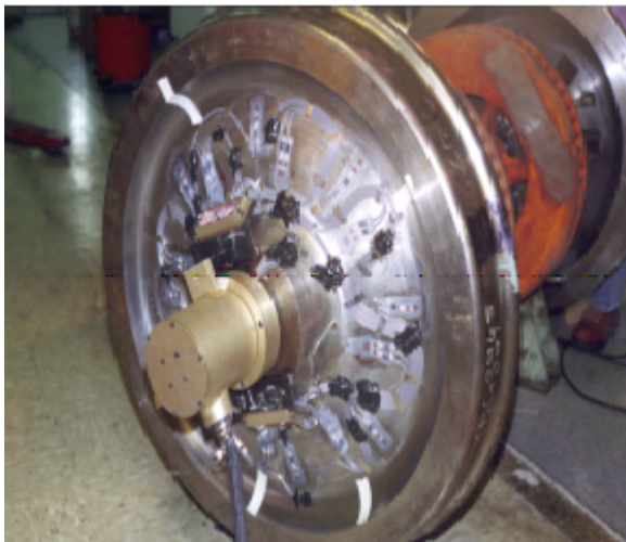
Figure 4. Instrumented wheels for measuring wheel/rail contact forces.
