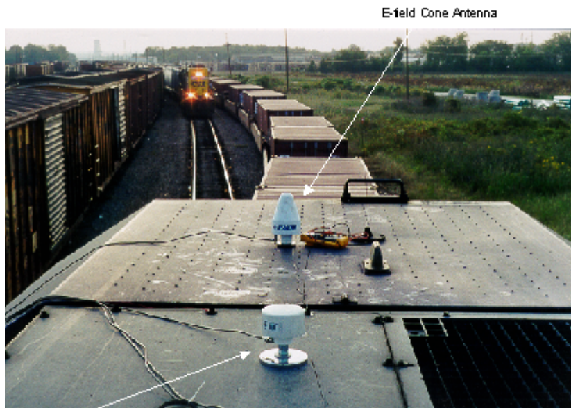
Figure 1. View of Starlink E-field and H-field Antennas Mounted on the Roof of a Locomotive.
