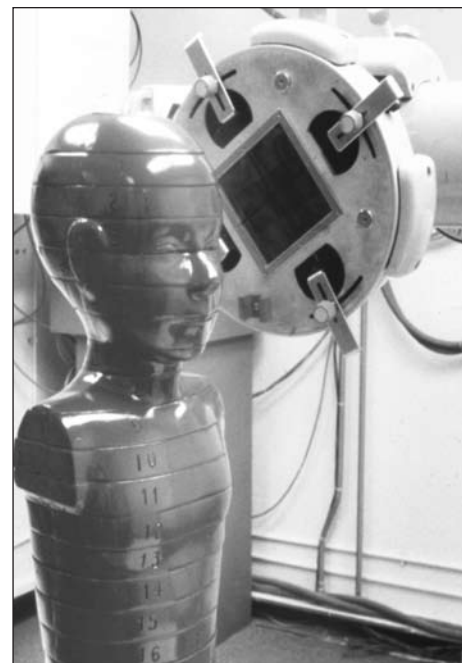
Left, a diagram of side view of tank of water in which dose rates are measured during exposure to x-rays to simulate scattering characteristics of human tissue. Right, a mannequin of a six-year-old child (made of material with a composition similar to human tissue) with imbedded dosimeters to help determine radiation exposures in real patients. (Both figures, Stovall M, et al. Radiation Res 2006;166:141–157)
