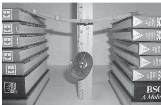
**Figure 2.4.** Testing the strength of bundled pasta.
