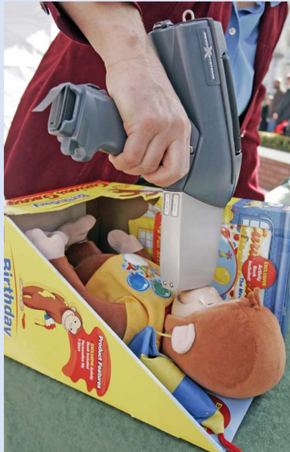
The exposure variable. A portable X-ray fluorescence analyzer can ascertain content of toxicants such as lead, arsenic, and cadmium (this toy had a reading of 6,253 ppm lead). It’s harder to tell, however, how much of any given toxicant is making its way into a child’s body.
