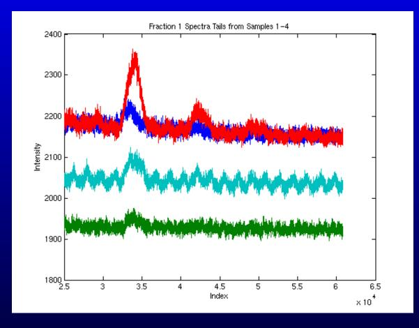
Roughly half the spectra have sinusoidal noise.
