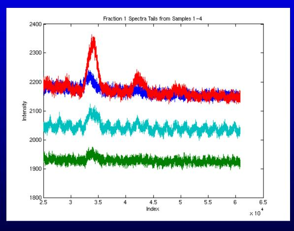
Roughly half the spectra have sinusoidal noise. We're seeing the A/C power cord.
