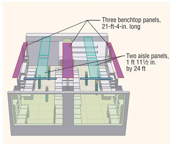
FIGURE 5. Two sets of ceiling-mounted cooling panels.
