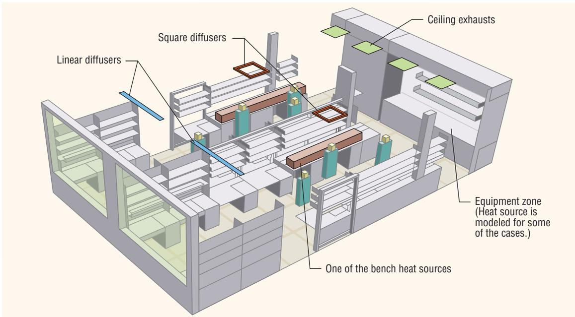
**FIGURE 1. Baseline laboratory-model layout.**
