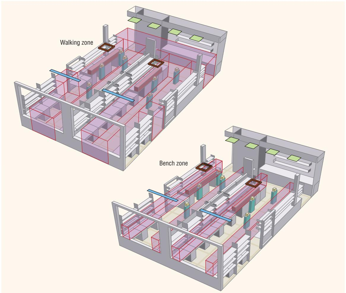
**FIGURE 2.** The walking zone included the red highlighted areas on the left figure. The bench zone included the volume above the benchtops in the red highlighted areas on the right figure.
