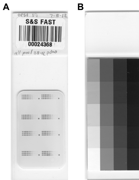
Figure 1. Reverse-phase protein lysate microarray (RPA) and wedge density strip (WDS). (A) RPA. Protein lysates from various cancer cell lines were mixed and spotted by a microarrayer (GMS417; Genetic MicroSystems/Affymetrix, Boston, MA, USA) onto glass slides embedded with nitrocellulose membranes. Each spot is approximately 600 \mu m in diameter. Each row represents one sample with 10 steps of a 2-fold dilution series. Therefore, theoretical protein concentration is log (base 2) scale from left to right. There are 24 rows on this array, all of which are the replicas. (B) The WDS mounted on a glass slide. There are 20 different sectors that differ in darkness from black to white. The optical density for each step in the scale was measured by reflective optical densitometry with a visual filter by the manufacturer.
