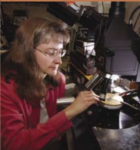
Mary Crawford tests the output of an ultraviolet light-emitting diode developed by a team that set new records for wavelength/power output.
