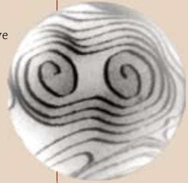
The dark bands are atomic steps on a TiO 2 surface as observed by low-energy electron microscopy. The closed islands are spawned from the two dislocation spirals. Field of view is 5 nm
