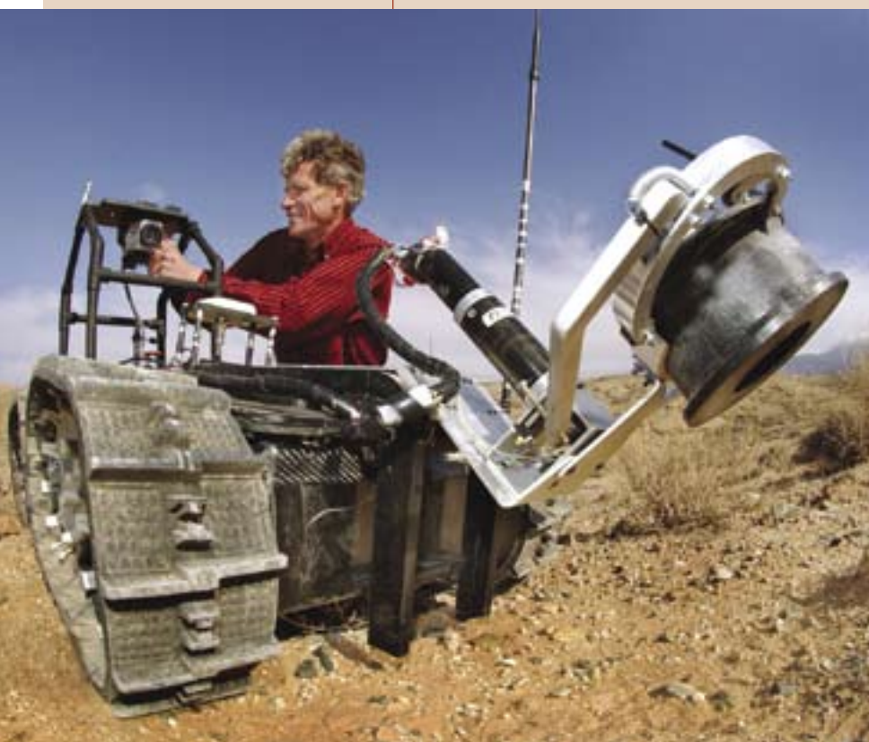
Alex Maish checks out SandDragon, developed for use in rugged outdoor terrain with two bodies, which push and pull each other over obstacles. SandDragon robots offer surveillance, reconnaissance, target acquisition, and response options in support of the military.
