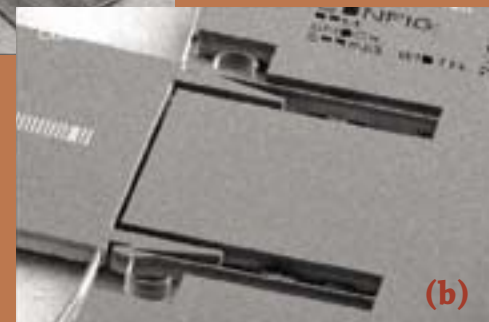
Microsystems-based safe-and-arm device; (a) safe position, (b) armed position.)
