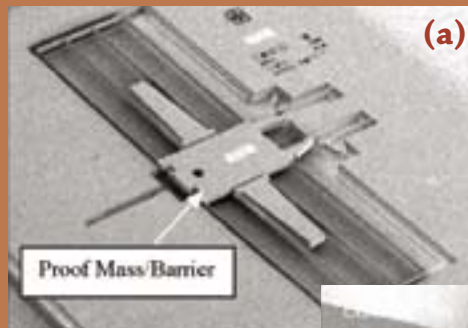
Microsystems-based safe-and-arm device; (a) safe position, (b) armed position.)
