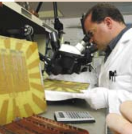
Todd Barnett inspects printed circuit board layers during the fabrication process at Sandia's Electronic Prototype Lab.
