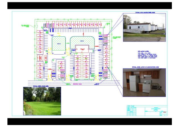
This is the design of a typical 50-units community site. It is projected that a typical unit should comfortably accommodate, on average, 2 - 3 individuals. The density of the site, defined as the number of individuals can be housed in the site at one time against the size of the site, is an important consideration during the community site design phase as the site density impacts site access as well as the size of each resident's individual lot.
