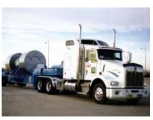
A legal-weight truck carries a cask containing spent nuclear fuel. Drivers are specially trained and certified, must be accompanied by at least one escort, must report in with the DOE every two hours, and are continuously monitored and tracked by satellite.
