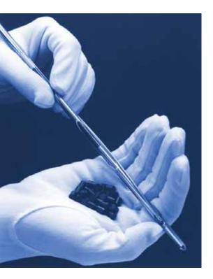
What is spent nuclear fuel? The fuel used in nuclear reactors is made of solid enriched uranium pellets about the size of a pencil eraser (shown above). Hundreds of these pellets are sealed inside strong metal tubes (fuel rods) that are bundled together to form a nuclear fuel assembly.
