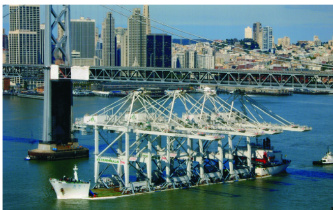
A barge loaded with four construction cranes passes underneath the Oakland Bay Bridge with two feet of clearance. State-of-the-art navigation tools, positioning information, and water level predictions from NOAA's National Ocean Service made this precise maneuver possible.
