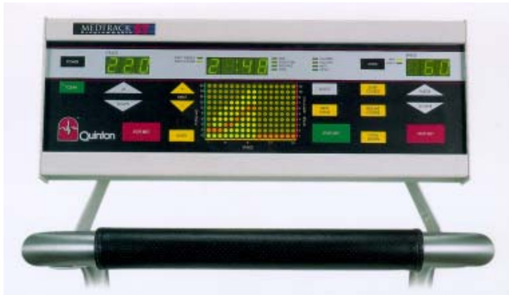
Figure 3-4. Treadmill controller - changing the exercise protocol
