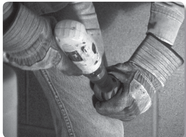
Solution: Using wire brush with power driver
