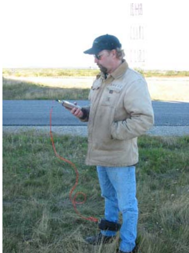
Photo 7: Ankle current measurement located directly beneath the lowest point of one of the main leads to the VLF antenna. Both feet are grounded.
