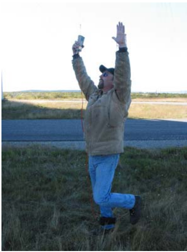
Photo 9: Ankle current measurement located directly beneath the lowest point of one of the main leads to the VLF antenna. Both arms raised while standing on one foot to maximize potential body current measurements.
