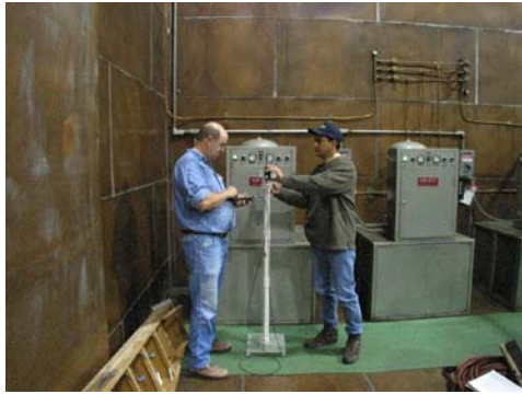
Photo 6: NIOSH investigators setting-up E-Field measurement located in the Combiner Room Entry (Copper Room) near the dry air compressor. (Note: Investigators were at least 4 meters from the instrument during measurements.)
