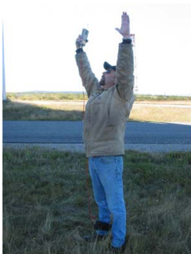
Photo 8: Ankle current measurement located directly beneath the lowest point of one of the main leads to the VLF antenna. Both arms raised to maximize potential body current measurements.
