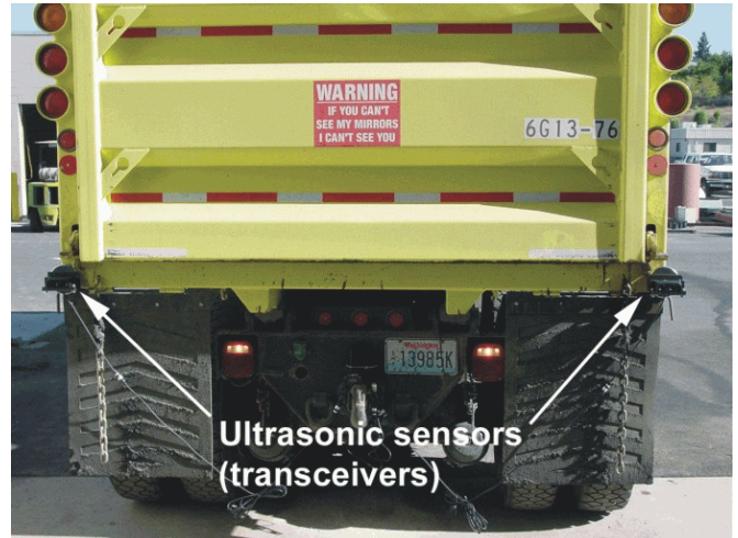
Figure 23.—Hindsight sensors mounted on dump box for short-term test.
