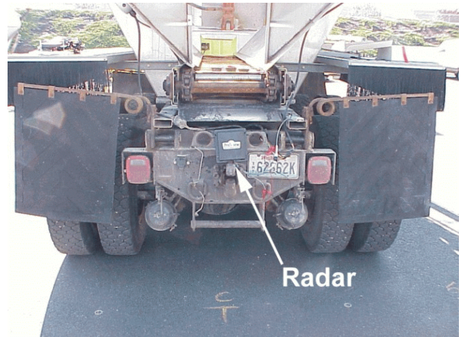
Figure 6.—Preview radar system temporarily mounted above hitch on sanding truck.
