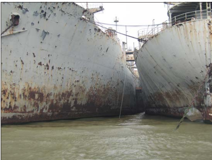
This is an example of the placement of mussel bags between the Reserve Fleet ships. The white rope seen to the left between the two vessels is attached to several mesh mussel bags.
