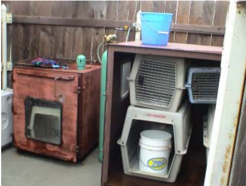
Figure 2. Large and small CO euthanasia chambers and associated CO supply system
