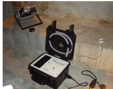
Photo 5: Upper left corner shows a Pylon ® radon monitor. Center shows a SKC Airchek HV30 Air Sampler and filter cassette, which is used to capture radon progeny. The filter is removed and the alpha disintegrations are recorded by a scaler counter.
