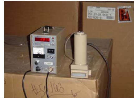
Photo 11: Ludlum Model 2000 scaler counter and Ludlum Model 43-10 detector used to count alpha activity on Teflon filters. The detector efficiency was 0.38 cpm / dpm.
