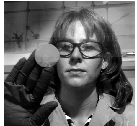
Tammy Taylor of the Laboratory performs a swipe on a surface potentially contaminated with beryllium. Taylor has developed a beryllium detection technique using colorimetric analysis.
