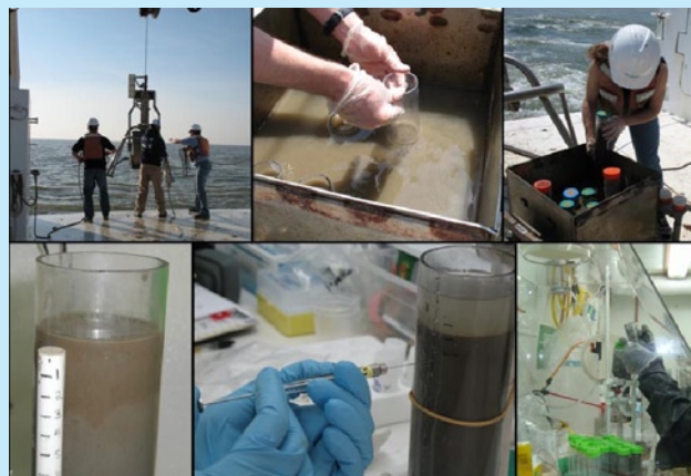
Clockwise from top left. Collecting boxcores in the Gulf of Mexico aboard the R/V Pelican. Subsampling boxcores, and removing sub-cores for processing in the R/V Pelican laboratory. Sectioning a core in an oxygen-free glovebox to separate porewater and solids. Injecting with an enriched isotopic mixture of inorganic mercury and methylmercury to measure methylation and demethylation rates. Oxygenated, brown sediments were evident in the top few centimeters at some stations. Photo credit: D. Senn
