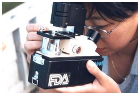
Figure 4. Volunteer observing plankton in the field portable microscope to determine if harmful algae species are present.
