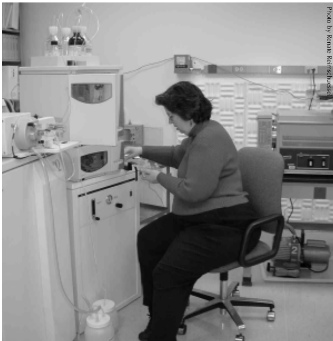
CVM chemists are evaluating triple quadrupole mass spectrometry for the confirmation of chloramphenicol residues in shrimp and honey.
