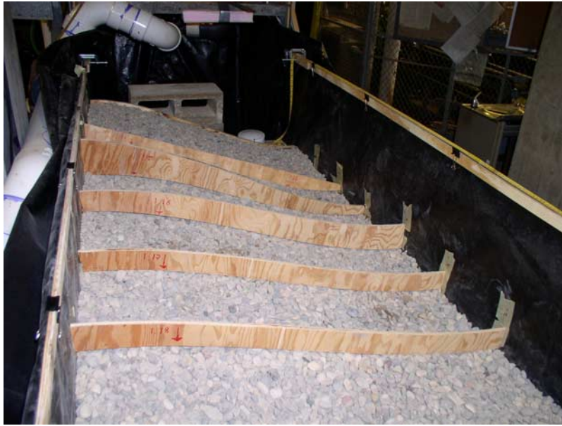
Figure 3. Process of pool-riffle construction using wooden ribs to mold bed topography.
