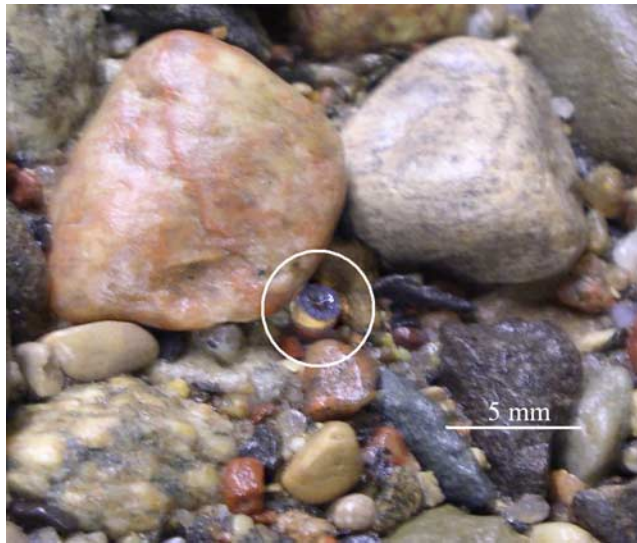
Figure 7. Photograph of a micropiezometer for measuring pressure at the sediment-water interface.
