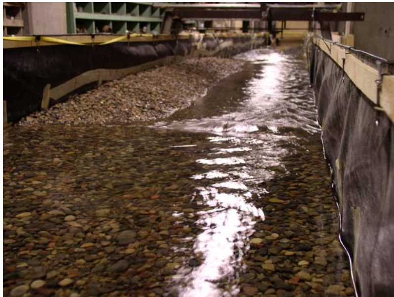
Figure 1. Example of low-flow experimental conditions: Exp1, 12.5 \text{ l s}^{-1} discharge, 0.0041 \text{ m m}^{-1} slope.
