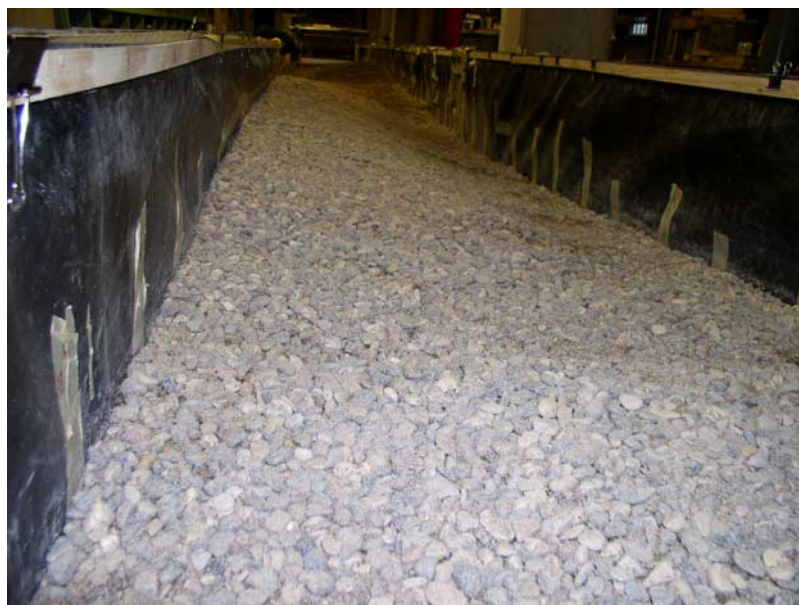
Figure 2. Pool-riffle bed form, with an amplitude-to-wavelength ratio ( \Delta/\lambda ) of 0.0215, largest amplitude.
