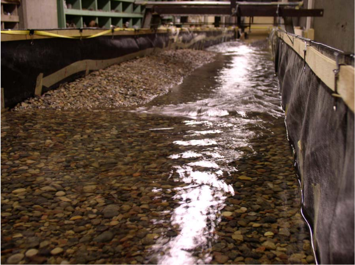
Figure 2.1: Example of low-flow experimental conditions: exp6, 12.5 \text{ l}\cdot\text{s}^{-1} discharge, 0.0041 \text{ m}\cdot\text{m}^{-1} slope.
