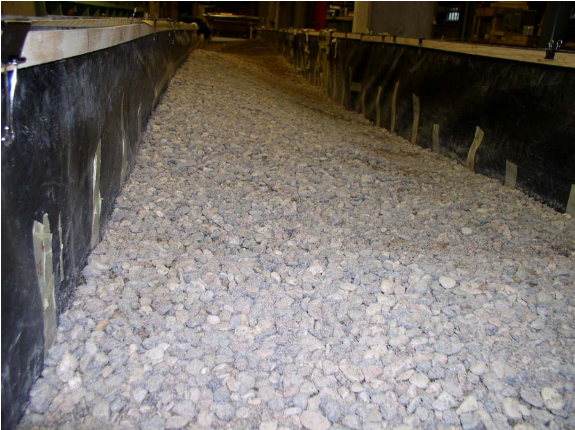
Figure 2.2: Pool-riffle bedform for ratio of bedform amplitude to wavelength ( \Delta/\lambda ) of 0.0215, largest amplitude.
