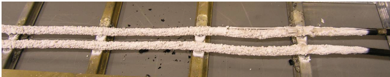
Figure 5.27: Post test photo of the SR cables following a Penlight test. Note that the cable did not fail in this test (PP-10).
