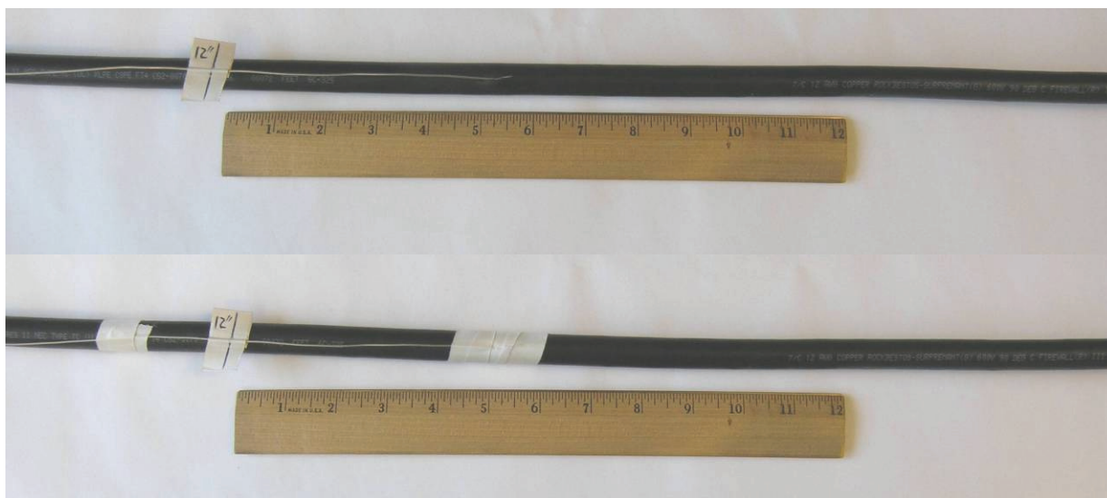
Figure 3.3: Illustration of a sheathed TC inserted under a cable's jacket.
