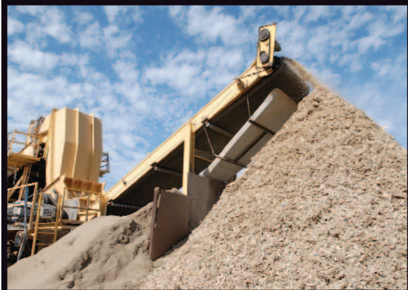
Wood I recycle if I could? If scrap wood can't be used architecturally, it can still be chipped for mulch, boiler fuel, or wood composite fodder.
