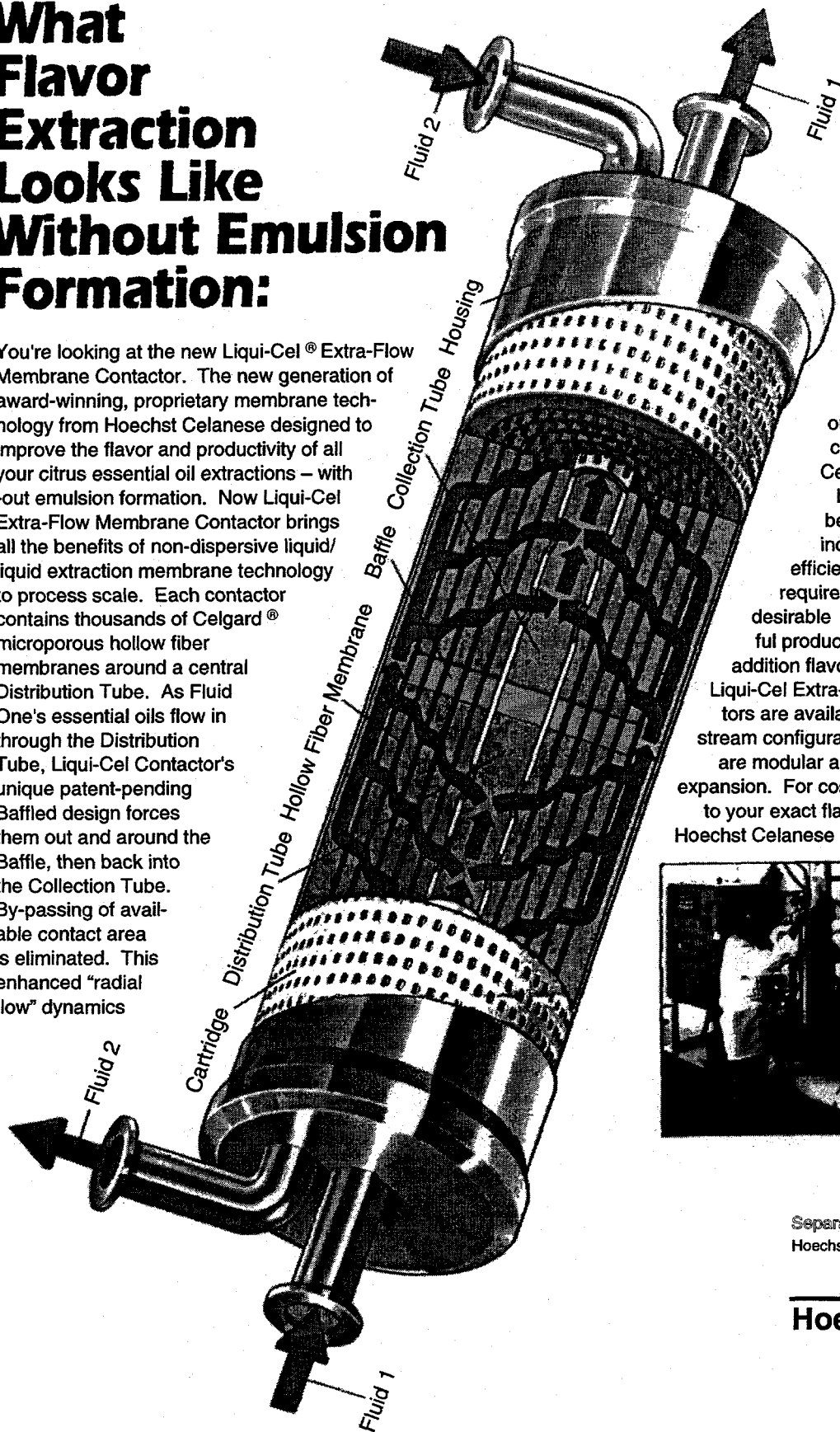
Figure 4-4. Flow pattern in new Hoechst/Celanese crossflow module.
