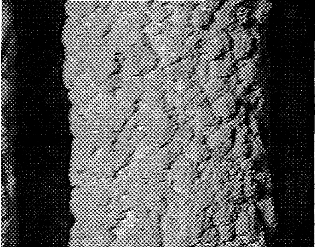
Figure 4. A representative photograph of the appearance of one of the lumpier filter cakes observed on a 3M filter element in the Westinghouse FL0301 filter at the PSDF on January 20, 1998.
