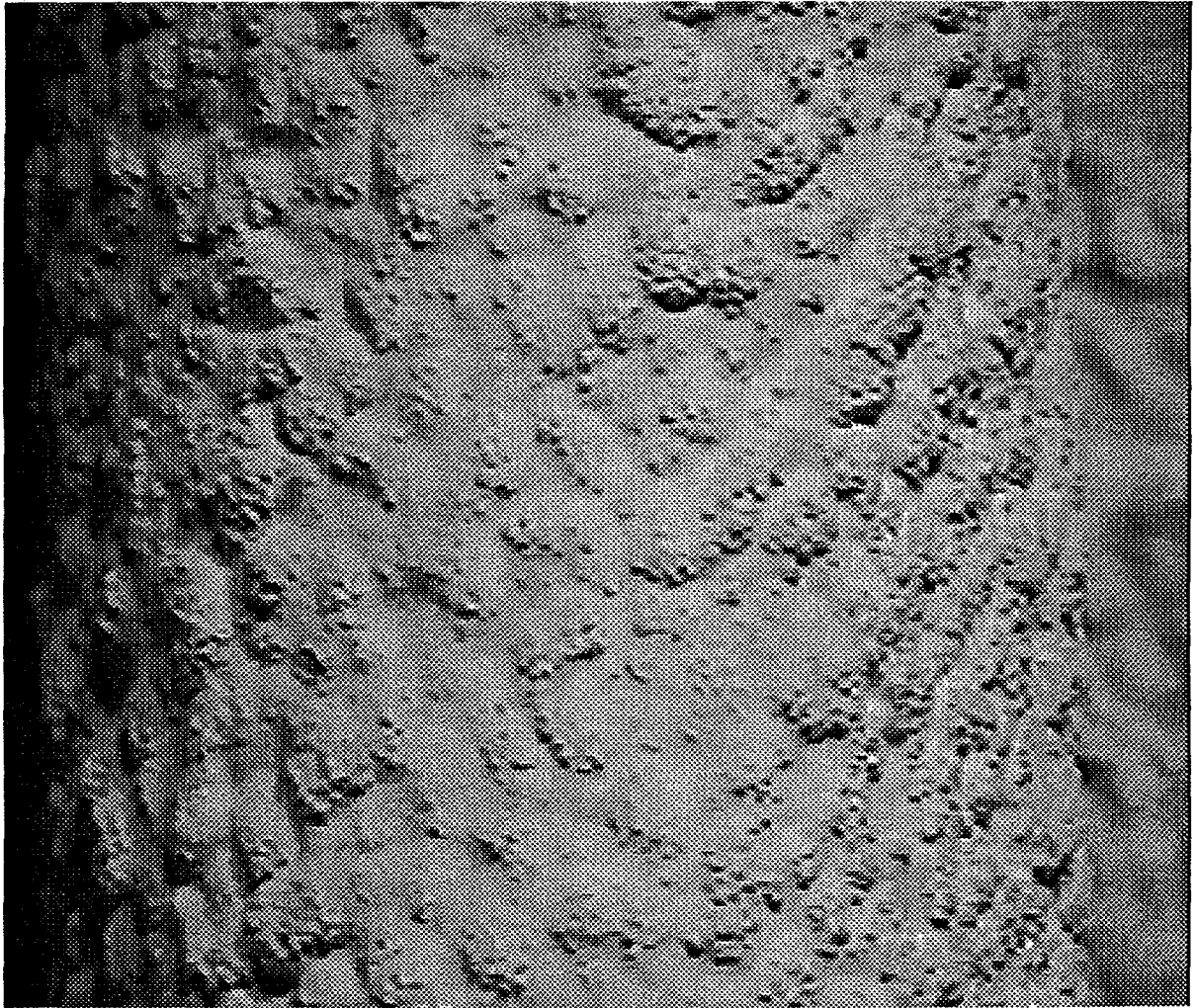
Figure 5. A representative photograph of the appearance of a relatively smooth filter cake observed in the Westinghouse FL0301 filter at the PSDF on January 20, 1998.
