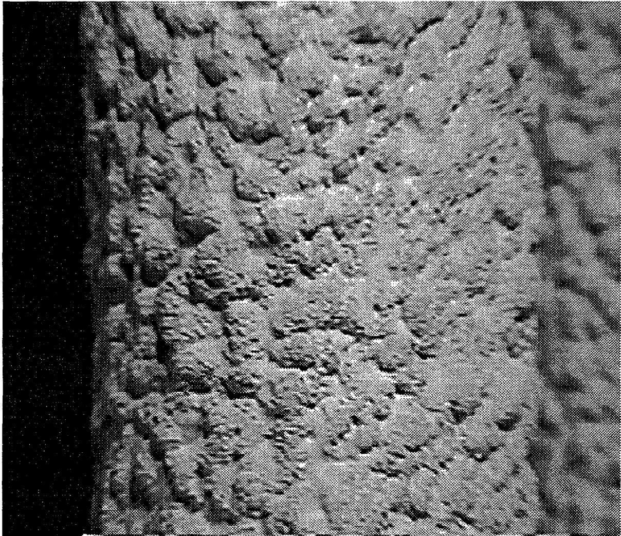
Figure 3. A representative photograph of the appearance of the majority of the filter cakes observed in the Westinghouse FL0301 filter at the PSDF on January 20, 1998.
