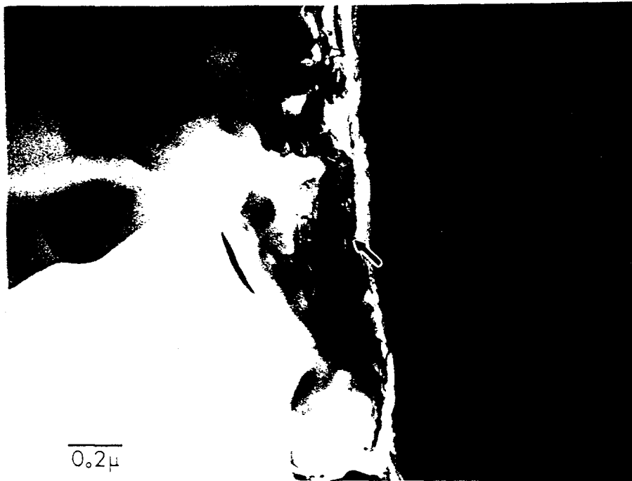
Figure 47. Transmission electron micrograph of NICALON fiber/SRSN interface. Graphite interface shown at arrow.
