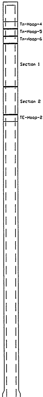
Figure 8. Cutting plan for Schumacher candle 344E-309.
