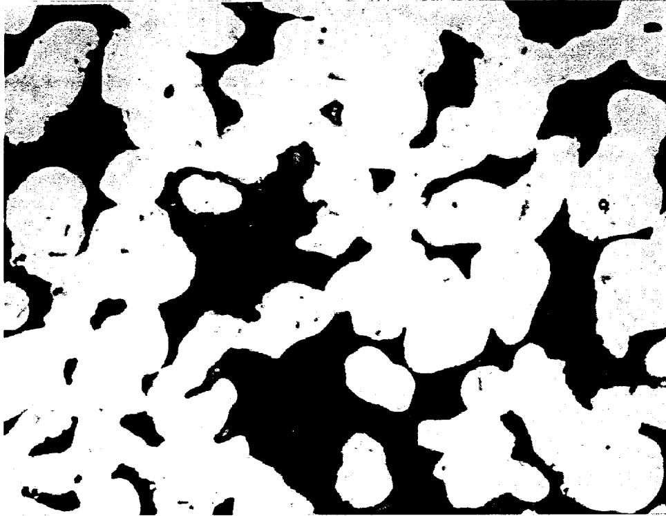
Photograph 3a. Photomicrograph of unexposed 310SC in the polished condition (400X)
