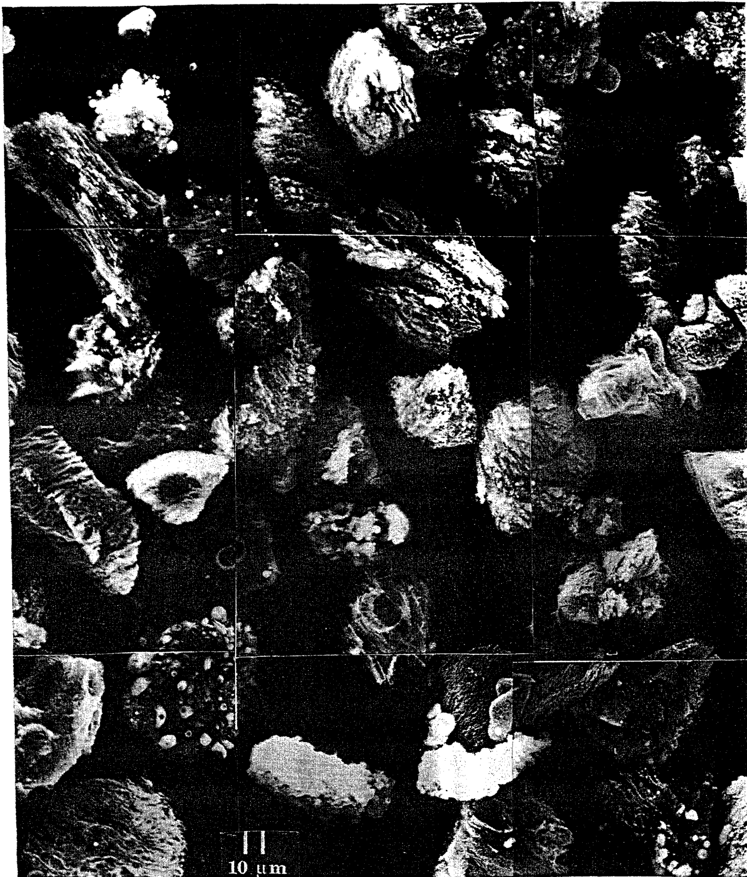
Figure II.D.1-4. SEM Microphotograph of Cyclone Fraction of In Flame Collection for Rosebud Coal. Magnification: X400.
