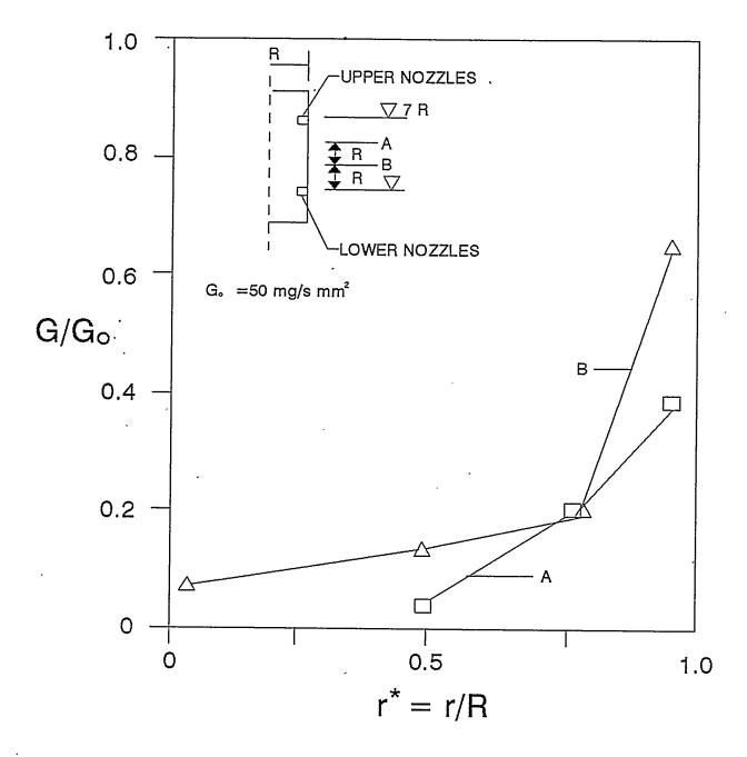
Figure 1 The Radial Distribution of Normalized Particle Mass Flux in the Exploratory Model
