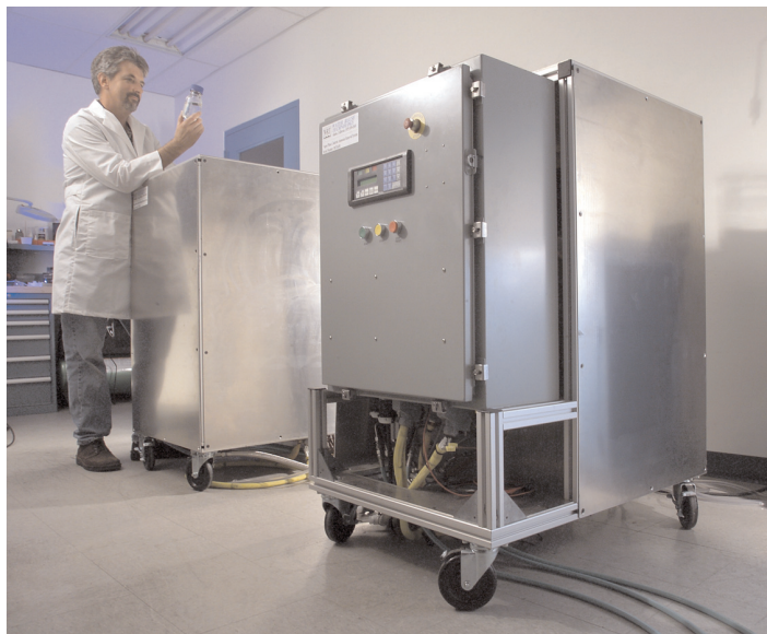
Space Drinks. (left) The photo shows two ARMS reactors which are currently being evaluated. It shows the teststand for the ARMS systems, which includes the reactor vessel and sensors. (right) VPCAR being tested in the lab.
