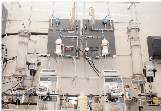
Space Drinks. (left) The photo shows two ARMS reactors which are currently being evaluated. It shows the teststand for the ARMS systems, which includes the reactor vessel and sensors. (right) VPCAR being tested in the lab.
