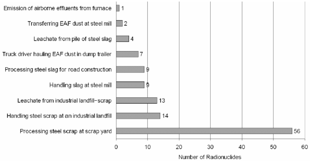
Figure E-1 Critical Group Exposure Scenarios and Defining Number of Radionuclides for the Release of Ferrous Metals
