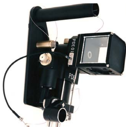
The dust chamber uses key components of proven USML flight hardware, TRL 9
