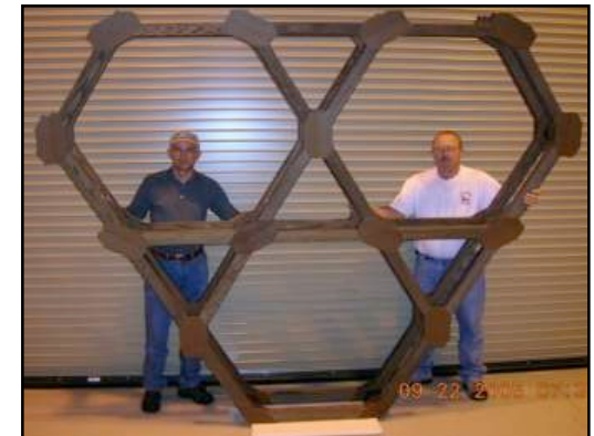
Completed fabrication of parts for cryogenic Backplane Stability Test Article and GSFC proved innovative metrology concept
