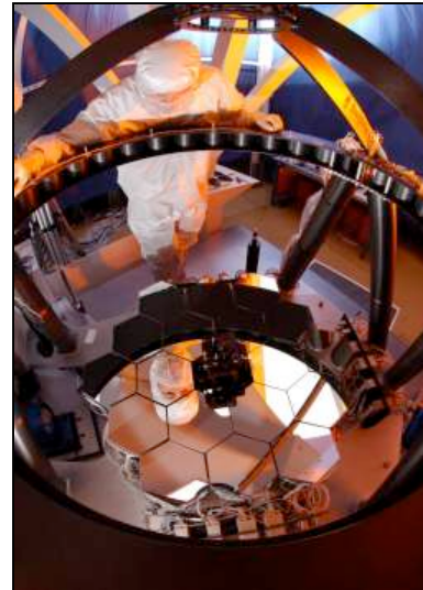
Completed 1/6 th scale Test Bed Telescope integration and initial alignment to prove wavefront sensing and control algorithms
