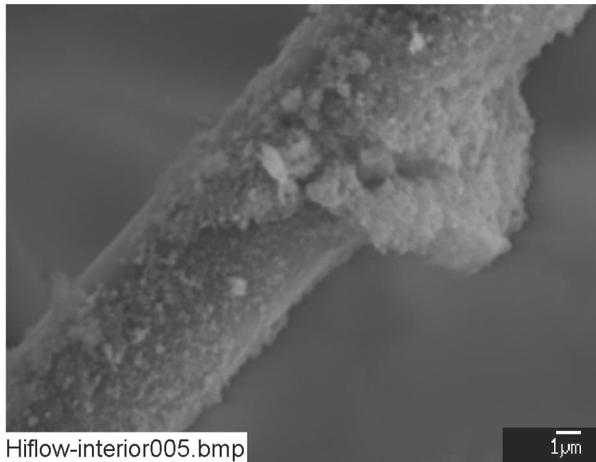
Figure D1-24. Test #2, Day-4 SEM image zoomed in on deposits on fiberglass, magnification 5000 times. (Hiflow-interior005)
