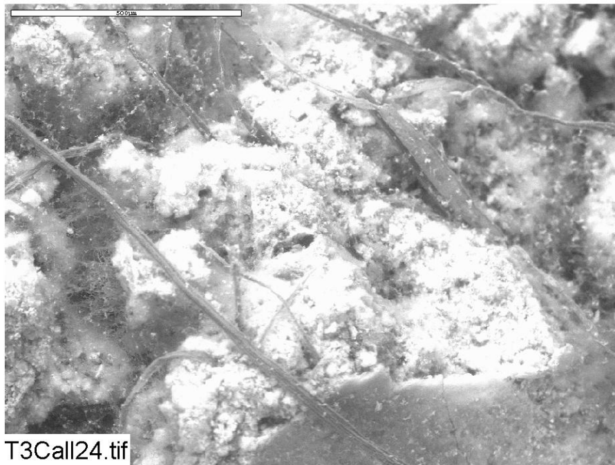
Figure H-15. ESEM image magnified 100 times for the interior of a Test#3, Day-30 raw cal-sil sample submerged in the birdcage. (T3Call24)
