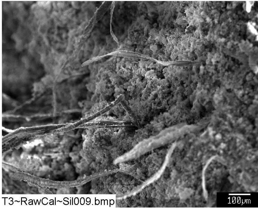
Figure H-7. SEM image magnified 100 times for a raw cal-sil sample. (T3~RawCal~Sil009)
