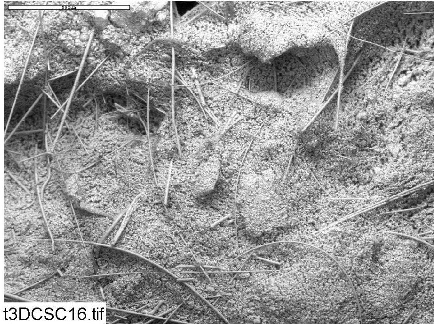
Figure C3-1. ESEM image magnified 100 times for a Test #3, Day-30 exterior fiberglass sample on the drain collar (adjacent to the drain screen). (t3DCSC16)
