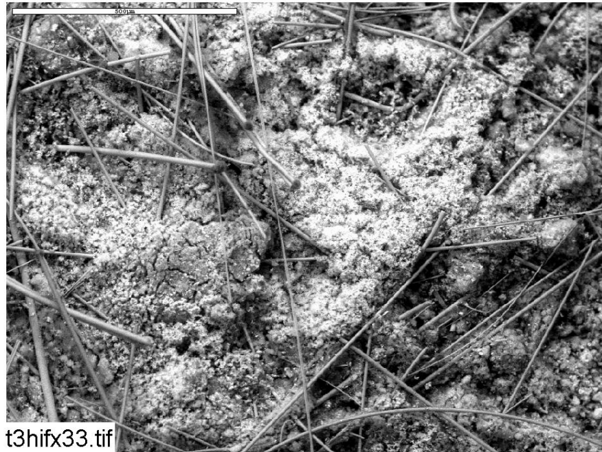
Figure C1-3. ESEM image magnified 100 times for a Test #3, Day-30 exterior high-flow fiberglass sample. (t3hifx33)
