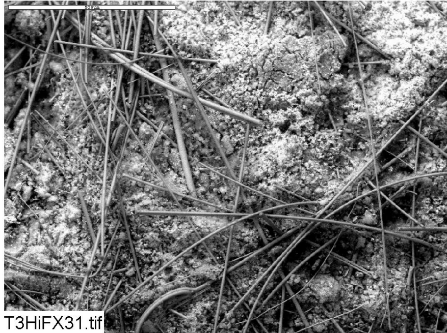
Figure C1-1. ESEM image magnified 100 times for a Test #3, Day-30 exterior high-flow fiberglass sample. (T3HiFX31)
