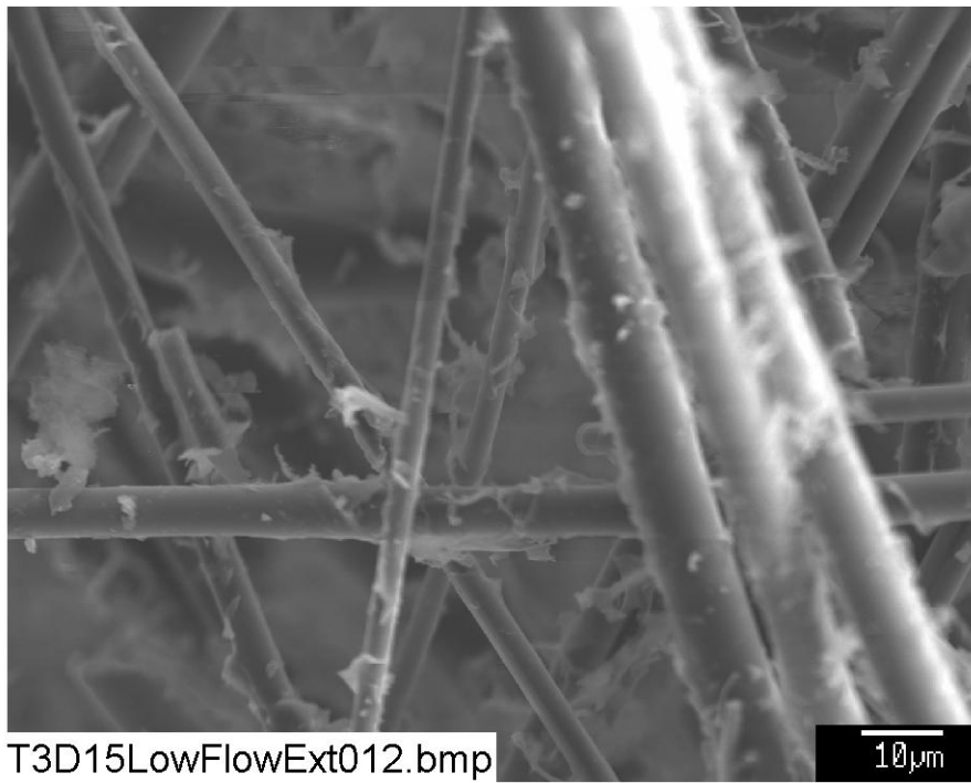
Figure B2-12. SEM image magnified 1000 times for a Test #3, Day-15 low-flow exterior fiberglass sample. (T3D15LowFlowExt012)
