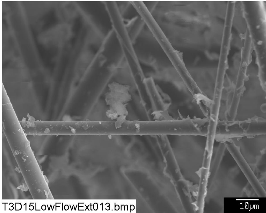
Figure B2-13. SEM image magnified 1000 times for a Test #3, Day-15 low-flow exterior fiberglass sample. (T3D15LowFlowExt013)
