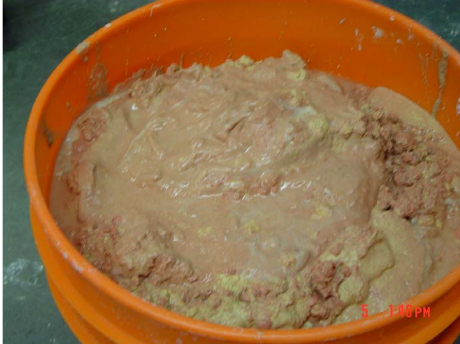
Figure 3-108. Sediment removed from the tank. Some gel appears on the top.
