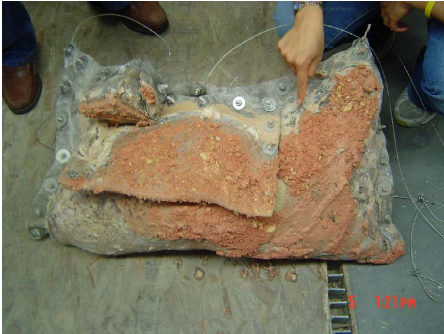
Figure 3-109. Samples removed from the tank bottom.
