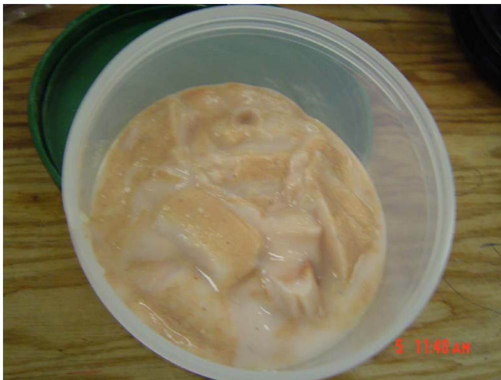
Figure 3-119. Gel-like material recovered from the bottom of the test tank.
