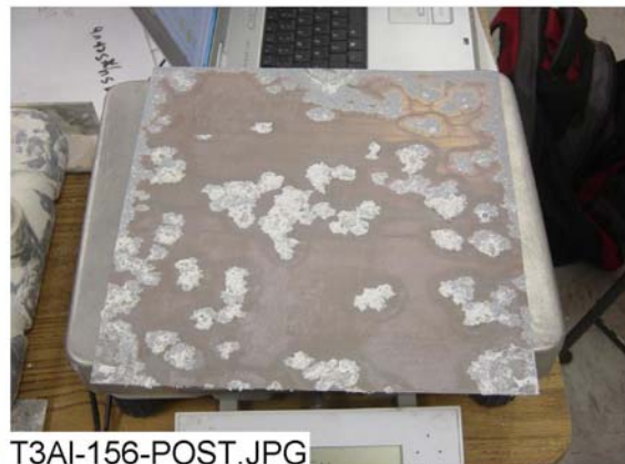
Figure 3-83. Al-156 submerged, post-test.
