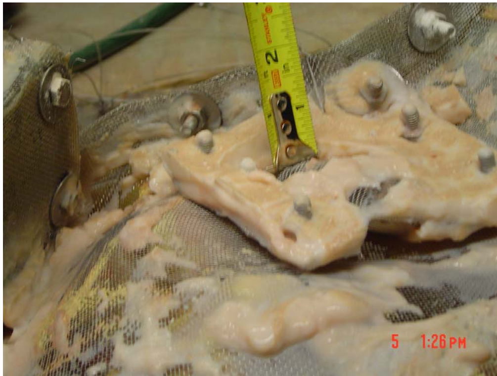
Figure 3-118. Gel-like material covering SS mesh on the bottom of the test tank.
