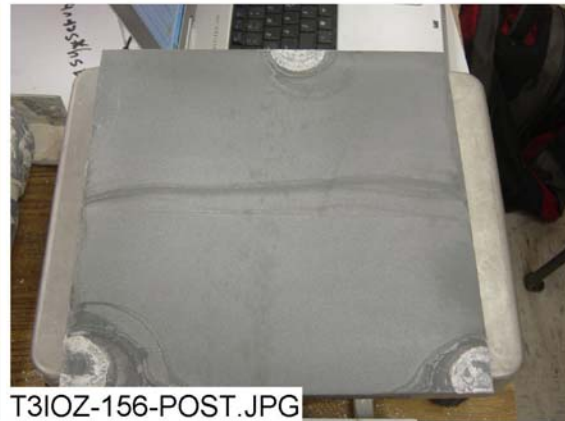
Figure 3-89. IOZ-156, submerged, post-test.
