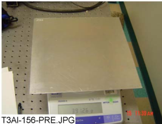
Figure 3-82. Al-156, submerged, pre-test.
